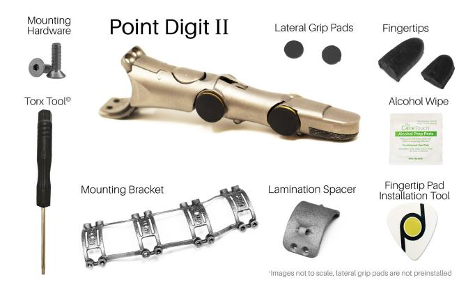
The **Point Digit** II is a passive (i.e. not powered) mechanical finger for people with partial hand amputation. It features a ratcheting mechanism that enables one-handed use and 11 distinct locking positions. The Point Digit II features integrated compliant touchscreen compatible\* fingertip pads for enhanced grip. The **Point Digit** II is made from titanium for ample strength.
