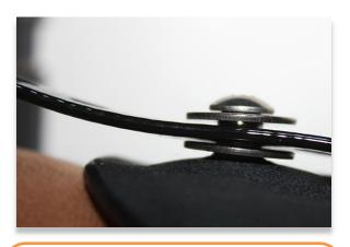
**Step 22:** Place one elbow strap washer between the strap and the forearm shell, and another washer on top of the strap before installing the retaining screw. Install screws on both sides of the elbow.
