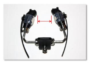
**Step 3:** Slip the HSC onto the user's arm above the elbow from the side. Ensure the space between the contacts is wide enough to pass over the upper arm from the side.
