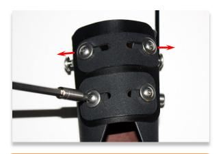
**Step 16:** Loosen the screws securing the width adjustment plates and spread the side shell pieces apart as wide as possible.
