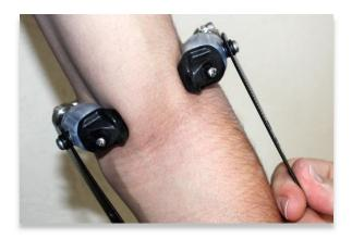
**Step 9:** Lightly pull down on the elbow straps to place a physical load on the HSC. *Note:* The HSC will stabilize at a fixed position on the arm. It should be possible to apply a substantial load without causing discomfort.
