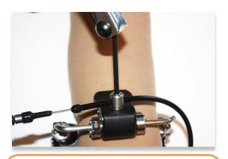
**Step 29:** Gently tighten the jam nut to lock the control cable position in the cable swivel. Large torque is not necessary to lock the cable in position. Avoid excessive torque to prevent damaging the cable housing.
