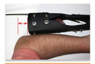
**Step 12:** Check for correct length. *Note:* The distance from the tip of the elbow to the rear edge of the width adjustment plate should be approximately 1" (2.5 cm).
