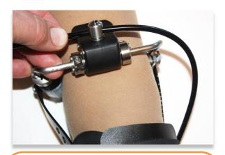
**Step 28:** Install the jam nut in the cable swivel on top of the compression washer. Position the control cable with sufficient length to allow for an ample loop around the elbow. *Note:* Users should be able to flex their elbow without an excessively large cable loop outside the elbow.
