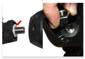
Step 31: Install the plastic washer between the terminal device and the distal cup of the forearm section. The conical spring washer is installed inside the end cup, with its convex side facing the hex nut. *Note:* If desired, removable thread lock compound or plumber's Teflon® sealing tape may be placed on the threaded post of the terminal device before installing the hex nut.
