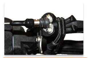
**Step 30:** Reattach the bent ball cable terminal to the terminal device.
