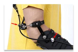
**Step 24:** The ITAL control cable attaches at two swivel points. One is located on the outer lateral side of the forearm. The other is located on the back of the HSC. *Note:* ITAL units ship with the cable attached to the forearm swivel only; the HSC is kept separate to facilitate fitting.
