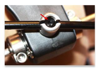
**Step 27:** Install the compression washer inside the cable swivel and touching the cable housing as shown.
