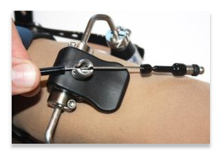
**Step 26:** Disconnect the control cable from the terminal device. Slide the cable housing cap towards the straight ball cable terminal and position the cable inside the cable swivel as shown.
