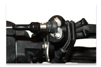
**Step 33:** Attach the control cable to the terminal device using the bent ball cable terminal. *Note:* This bend relieves flexing movements that place stress on the cable and preserves service life.
