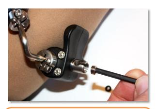
**Step 25:** Remove the jam nut and compression washer from the cable swivel on the back of the HSC and set aside. Use caution to avoid losing small parts.
