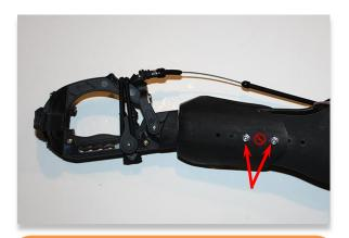
**Step 13:** Adjust length by selecting and matching holes in the forearm shells and distal cup. For maximum strength, two (2) screws should be installed per side with at least one hole separating them, not in adjacent holes.
