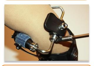
**Step 11:** Confirm all clamping collars on the HSC have been tightened to avoid inadvertent loss of adjustment.
