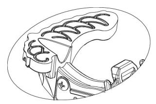
Tip Boot installed with securing tab removed.
