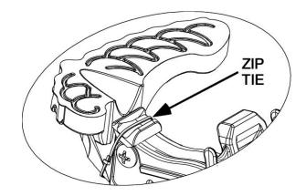
Optional methods of securing Tip Boots to the V2P using Rubber Bands (Left) or Zip-Ties (Right).
