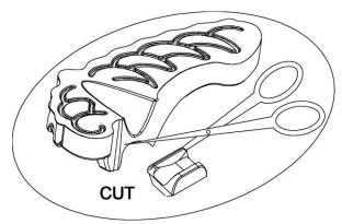
If desired, scissors or a sharp knife can be used to remove the securing tab.
